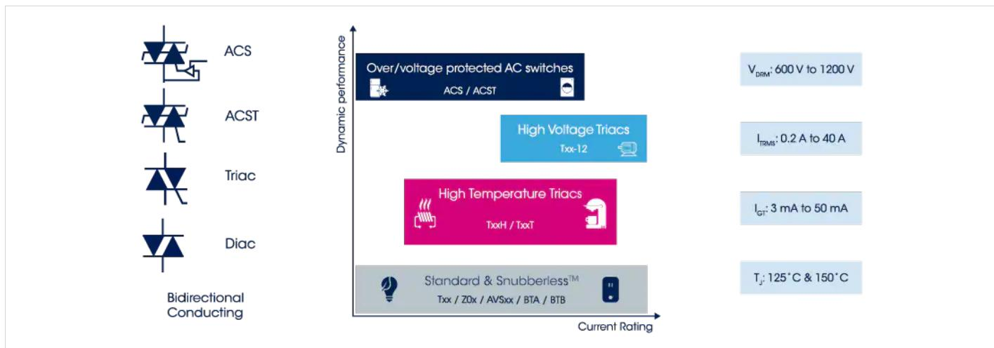
**Thyristors (SCR) and AC Switches / Triacs/Automatic voltage switches**
