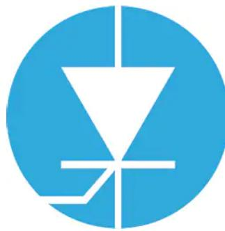
Silicon-controlled rectifiers (SCR) are the most immune switch to voltage spikes and their load commutation capability is very high.
