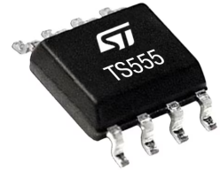
TS555: single CMOS timer with very low power consumption
