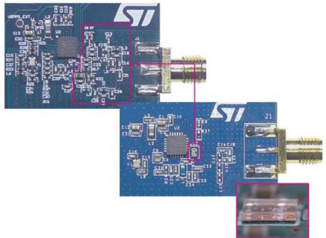
ST's IPDs available as standalone products such as baluns and filters as well as foundry services. They are compatible with different assembly modes, including CSP, microbumping, and wire bonding, for mounting on the main printed wiring board (PWB) or in a complete RF module.
